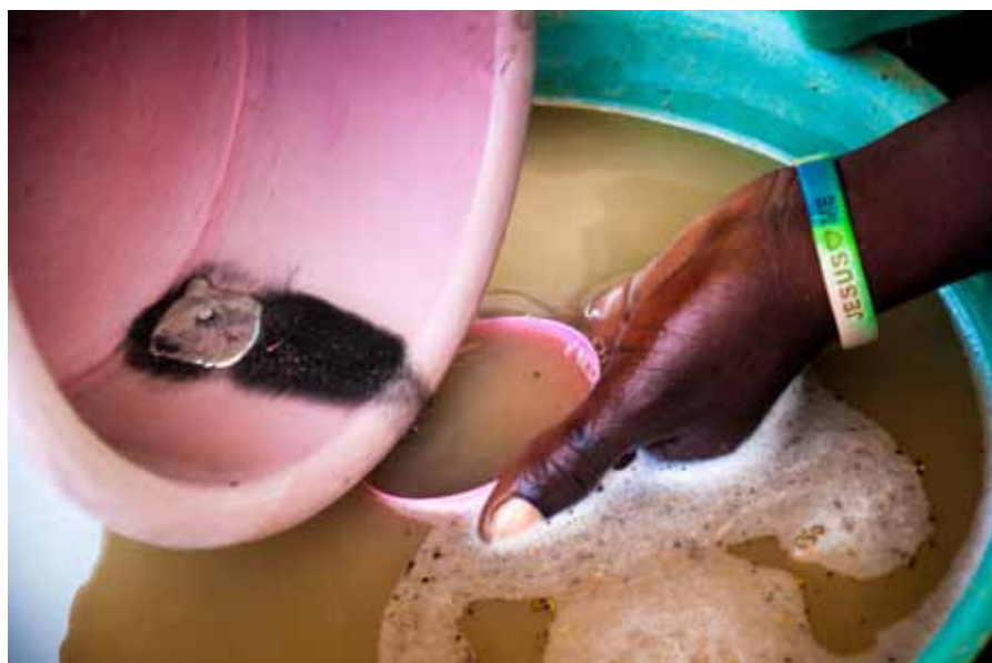
Figure 80: Initial steps of separating gold from ore using mercury (amalgamation)
