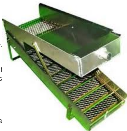
Figure 100: Typical sluice box
