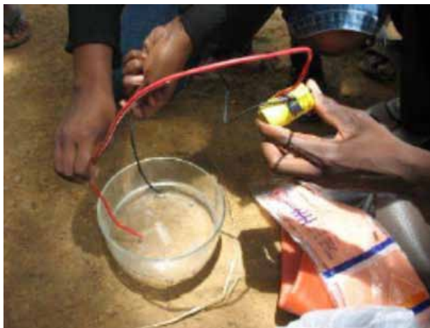
Figure 85: Miner activating mercury using a radio battery
