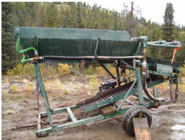
Figure 86: Mobile sluice box
