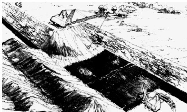
Figure 29: Strip mining with dragline on overburden and rope shovel loading coal below
