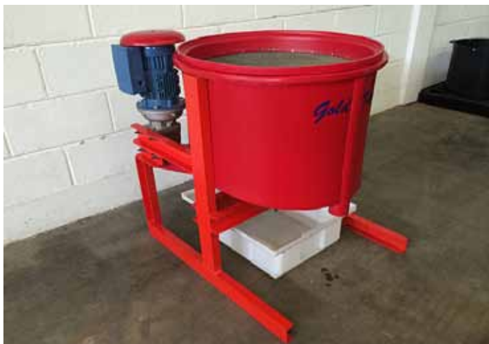
Figure 87. Centrifuge gold kacha, commonly used in Zimbabwe
