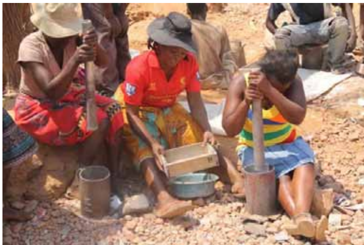
Figure 96: Mortar and pestle grinding in ASM
