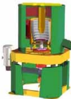
Figure 103. Knelson separator and Centrasep concentrator
